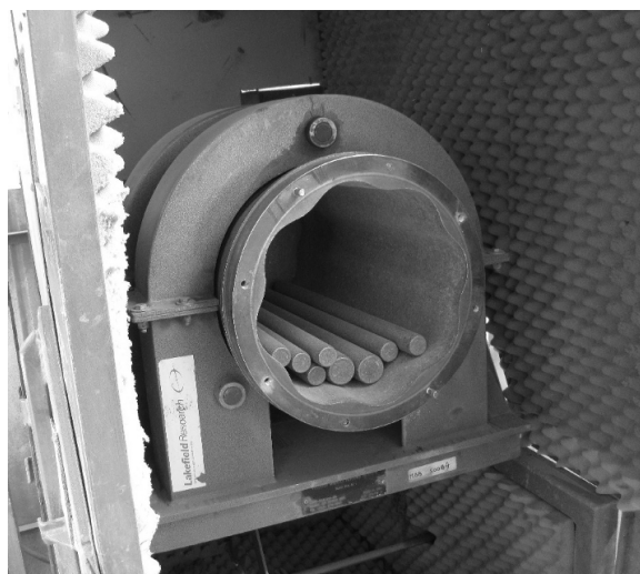
Figure 3: Rod mill for determining Bond rod mill work index
