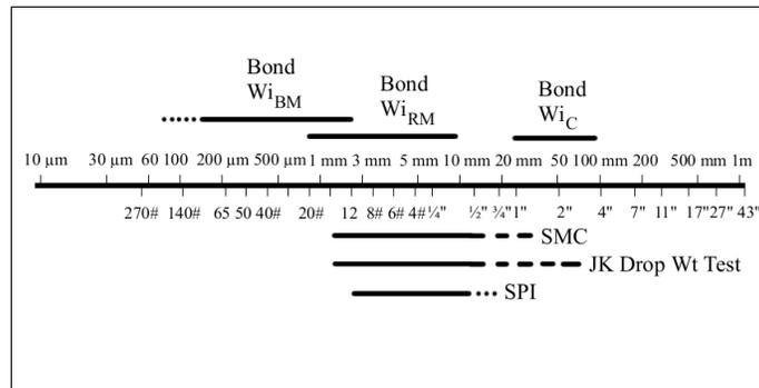
Figure 1: Size Ranges of Comminution Tests
