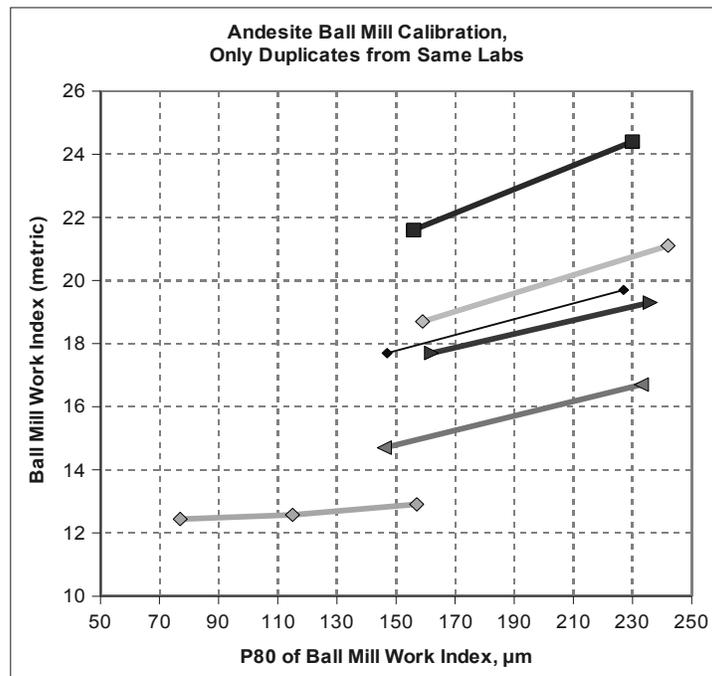
Figure 17: Variation in Ball Mill Work Index by Product Size for an Andesite Copper Ore
