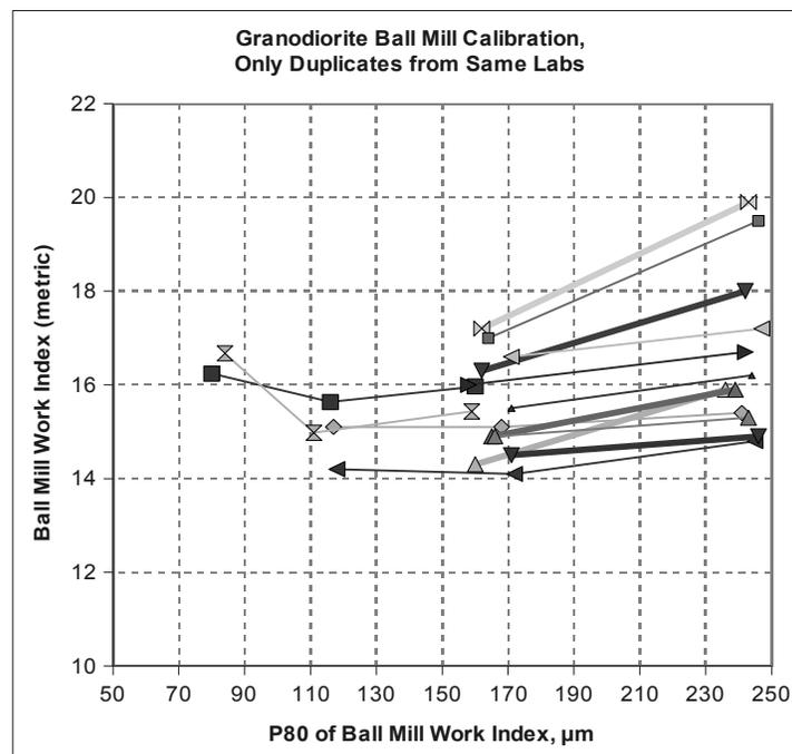
Figure 16: Variation in Ball Mill Work Index by Product Size for a Granodiorite Copper Ore
