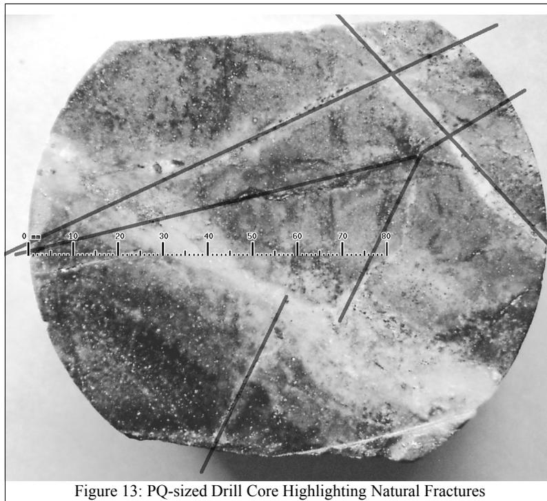
Figure 13: PQ-sized Drill Core Highlighting Natural Fractures
